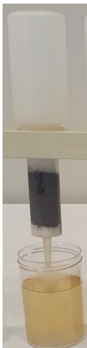
Figure 2. Soil column set-up
