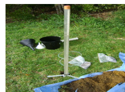
Figure 1: Schematic of a constant head permeameter
