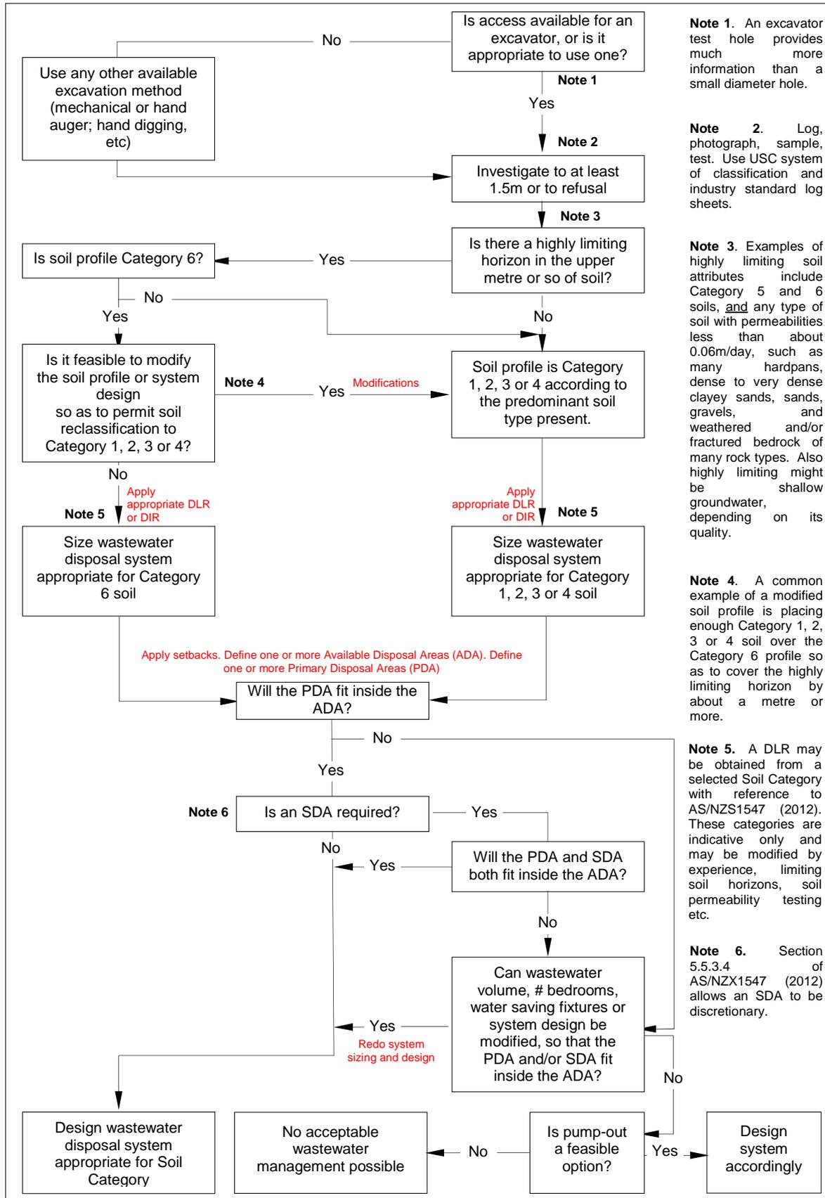
**Figure 4 Suggested flow chart for on-site wastewater assessment.**
