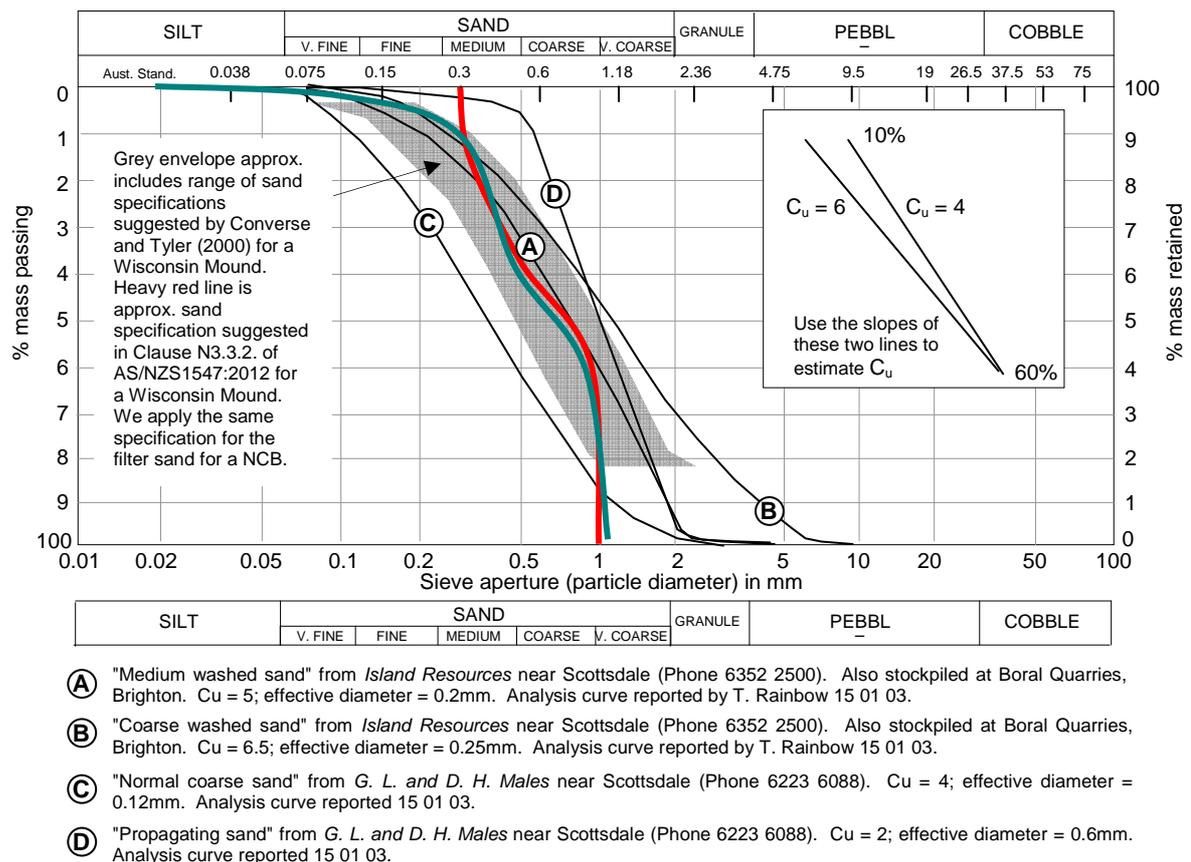
**Figure 6. Grain size curves for Tasmanian screened sand materials (slightly modified from Cromer, 2004). The red and green lines are two of a series of curves that comply with Clause N3.3.2 of AS/NZS1547:2012; in both cases, the  $C_u$  is about 3.3.**
