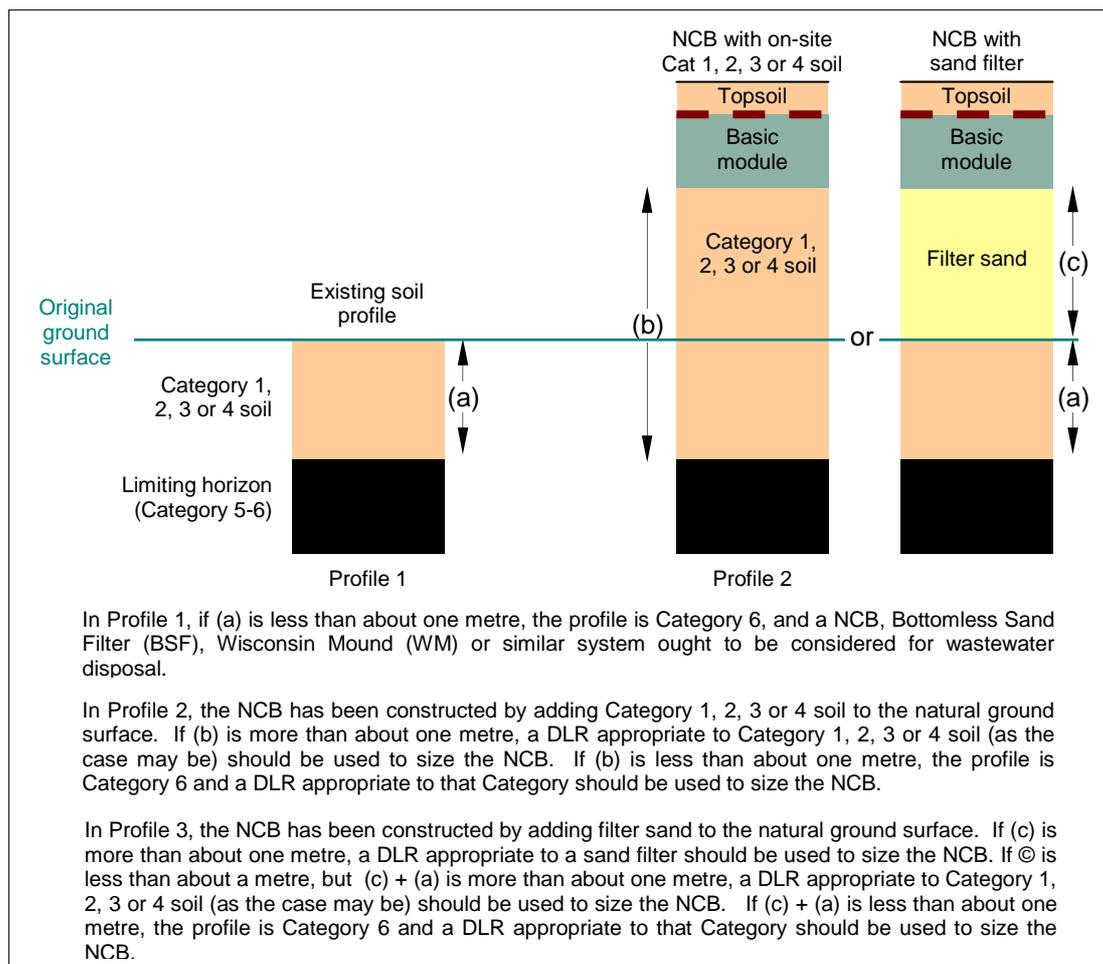
**Figure 8. The design loading rate (DLR) of an NCB, and hence the size of its basic module, is less than or equal to the loading rate of the least permeable soil in the first metre or so beneath the basic module.**
