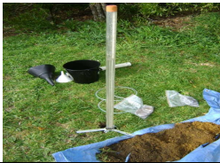
Figure 1: Schematic of a constant head tube permeameter
