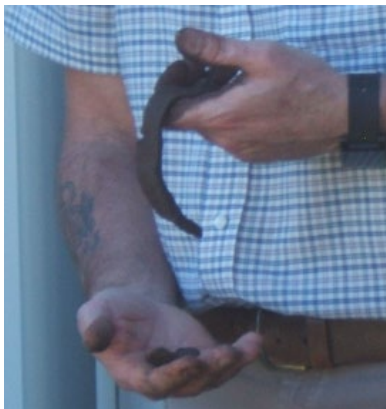
Figure 4. Forming a ribbon from the bolus
