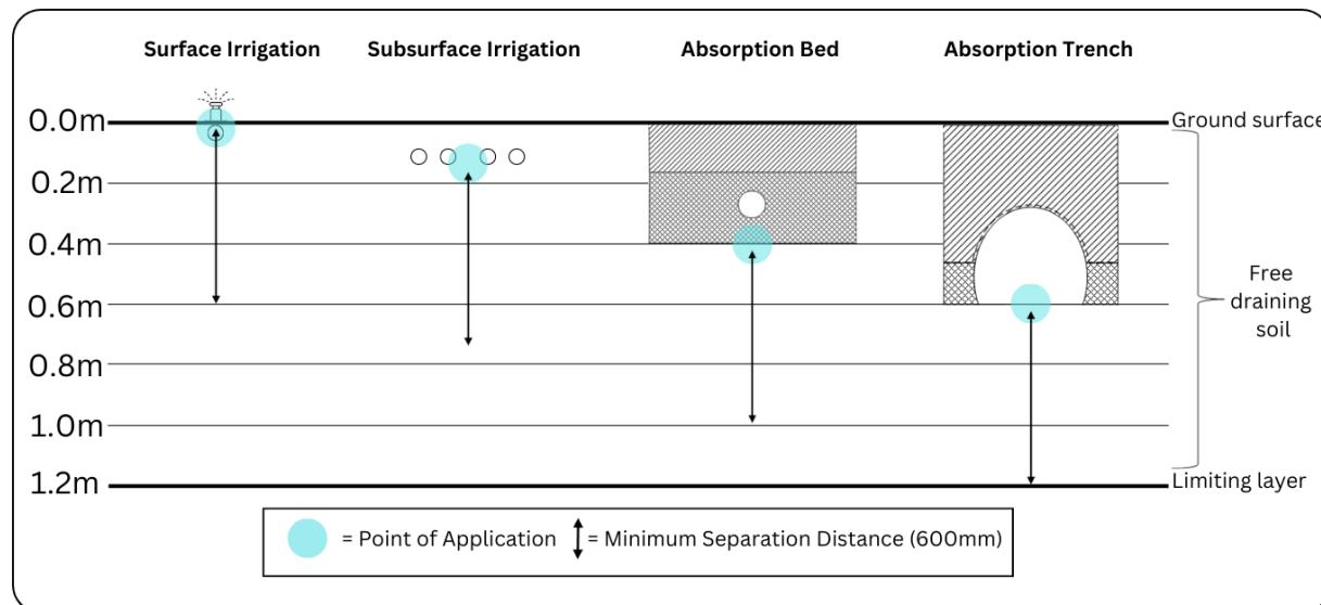
**Separation distance** – The separation between the point of application and a limiting horizon. The separation distance between the point of application and the limiting layer (or constraint) should be a minimum of 0.6 metre.
