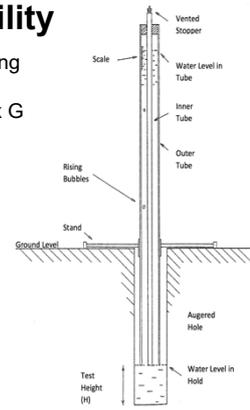
Figure 1: Schematic of a constant head permeameter
