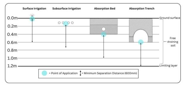
**Separation distance** – The 'vertical' separation between the point of application and a limiting horizon. The separation distance between the point of application and the limiting horizon (or constraint) should be a minimum of 0.6 metre.
