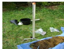
Figure 1: Schematic of a constant head tube permeameter
