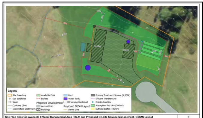
Site Plan Showing Available Effluent Management Area (EMA) and Proposed On-site Sewage Management (OSSM) Layout
