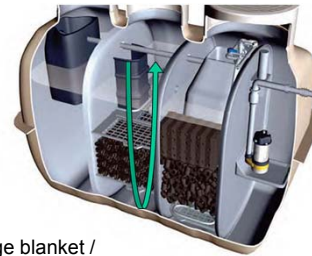
Up-flow sludge blanket / fixed-bed process e.g. FujiClean CE1500
